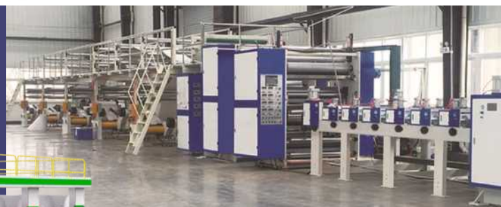
4/5/6 PLY KAPPA BOARD PRODUCTION LINE
